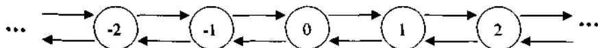
Figure 2.4. Unrestricted random walk; the probability of moving right is p and left is q .
